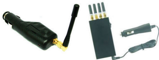
Figure 1: Typical portable GPS jammers powered by vehicle cigarette lighter ( http://www.insidegnss.com/node/2031 )
