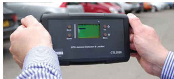
Figure 2: Handheld GPS jammer detector ( http://gpsworld.com/chronos-releases-handheld-gps-jamming-detector/ )
