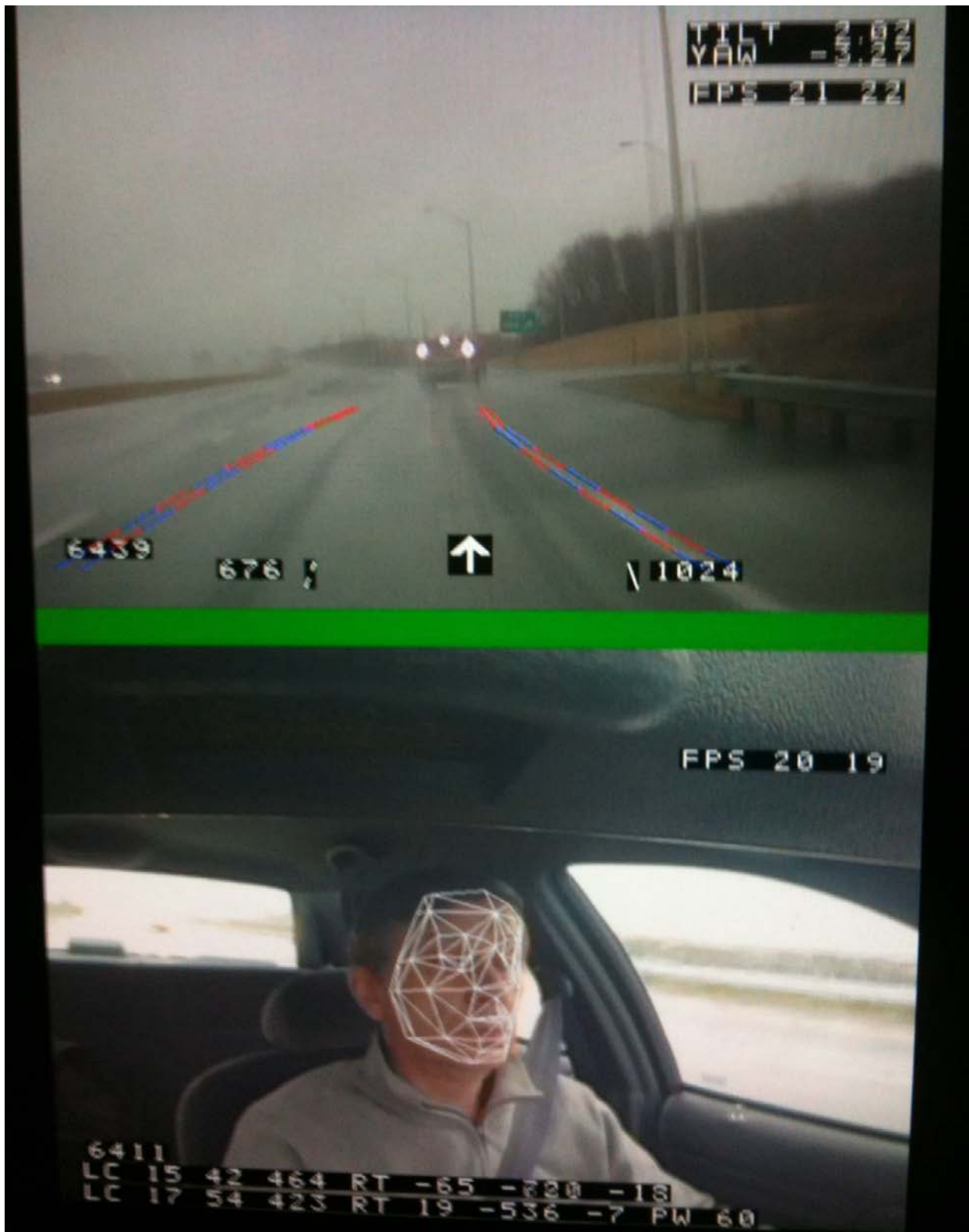
FIGURE 6 Screen capture of “Road Scout” lane tracking and “Mask” head position software operating on the DRIVE-SMART prototype system.
